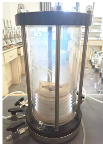
Fig. 2. Modified flexible-wall permeameter
